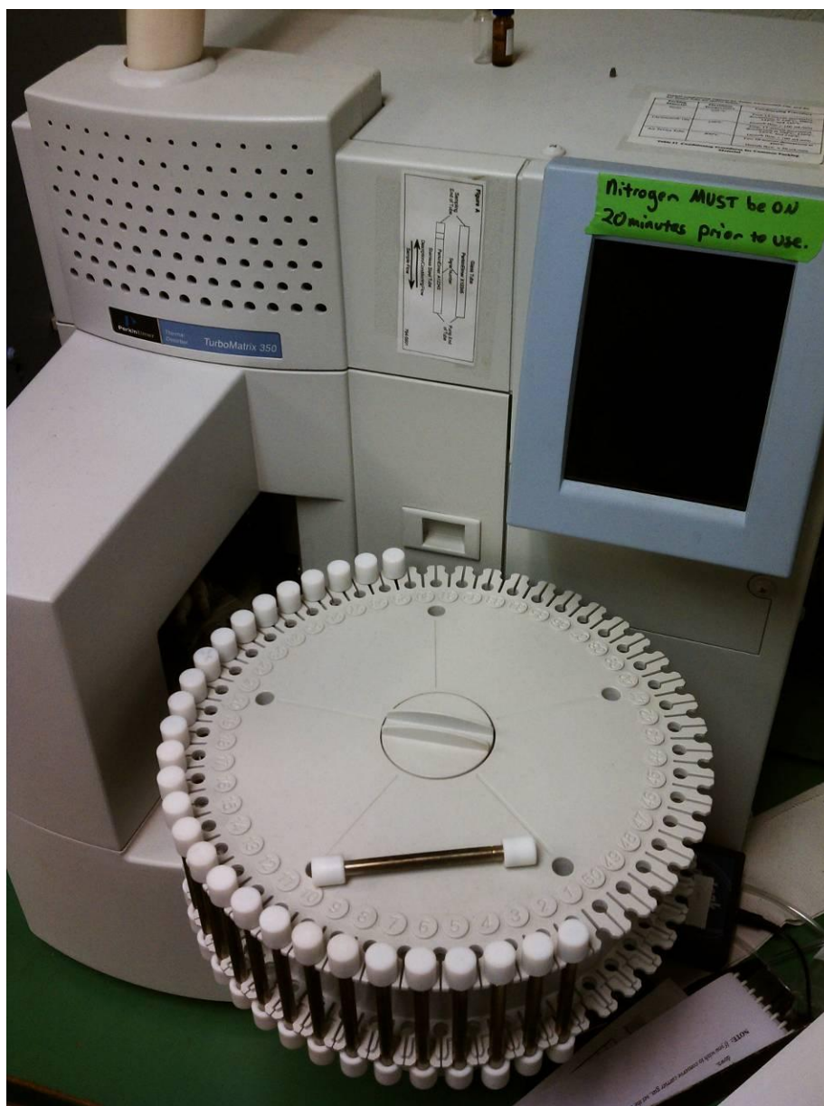
Figure 3 Perkin Elmer Automatic Thermal Desorption Tube and Carousel.
