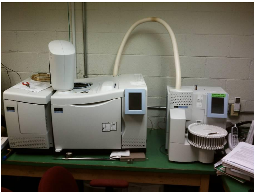
Figure 16 Setup for authentic science inquiry, using ATD GC-MS
